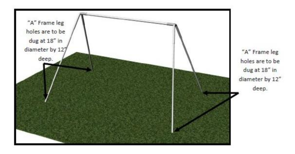
Place the set into the holes. Align the legs.
