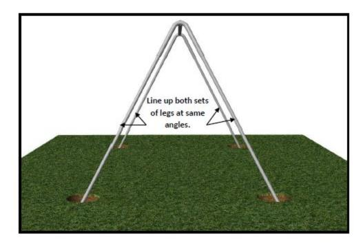
Place a level on the top rail and make the necessary adjustments to get set level.
